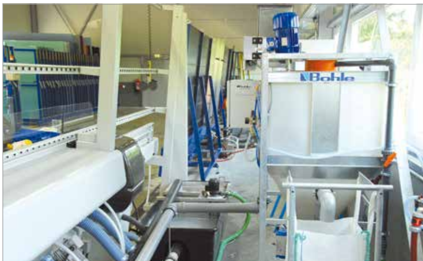
"The particle removal, cooling and service lives of the abrasive belt are significantly improved by clean cooling water and the reduced pollution translates into simplified cleaning for the entire system" reports the Egger Glas machine operator.
