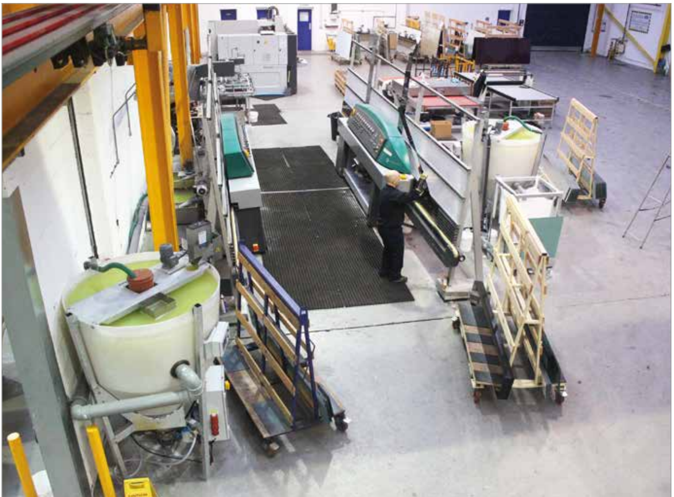
Wholesale Glass have installed a dedicated Sedimentor 1.0 on each of their Bottero straight line edgers which has increased productivity by more than 10%.
