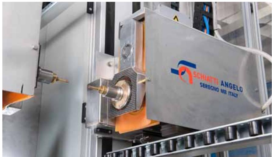
**The displacement of the spindles on Y axis (vertical movement) and Z (in and out movement) is carried out along ball-guides and screws,** which are protected with pressurized covers so that the air doesn't allow to outer agents, like water, powder etc., to go inside. The screw-support system allows a high displacement speed (up to 30 m/min).
